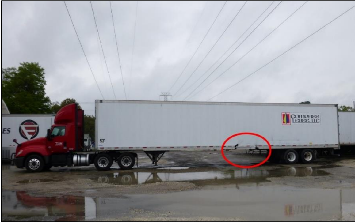
Figure 4. Left side of combination vehicle. Damage to lower edge of semitrailer sidewall rails is circled in red.
